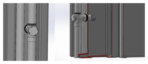
\*Warning\* Correct hole saw sizes must be used for the wallace seals provided to avoid leaks.
